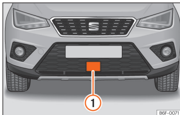
Fig. 145 On the front bumper: radar sensors.
