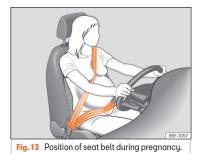
Seat belts offer their maximum protection in the event of an accident and reduce the risk of sustaining severe or fatal injuries only when they are properly positioned. Furthermore, if the webbing is correctly positioned, the seat belt will hold the vehicle occupants in the optimum position to ensure the airbag provides the maximum protection. The seat belt must therefore always be worn and the webbing correctly positioned.
