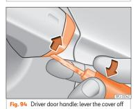
If the central locking system should fail to operate, the driver door can still be locked and unlocked by turning the key in the lock. As a general rule, when the driver door is locked manually all other doors are locked. When it is unlocked manually, only the driver door opens. Please observe the instructions relating to the anti-theft alarm system **»** page 106.
