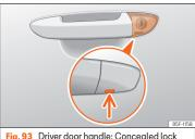
Fig. 93 Driver door handle: Concealed lock cylinder.
