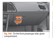
Depending on the vehicle's equipment, the CD player and SD card reader are located in the glove compartment.
