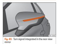
The side turn signals are LEDS and are integrated in the rear view mirrors.
