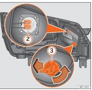
Fig. 56 In the engine compartment: main beam headlight bulb (2) and turn signal bulb (3).
