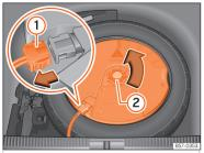
Fig. 234 In the luggage compartment: remove the subwoofer.
