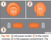
console, (2) in the luggage compartment. The USB power socket is located at the rear of the centre console (3).
