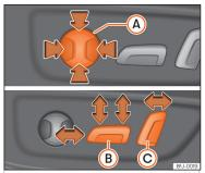
Fig. 118 Driver's seat: electric seat settings.
