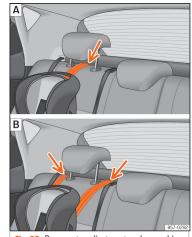
**Fig. 28** Rear seats: adjustment and assembly according to the Top Tether belt.
