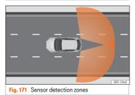
The radar sensors are located on the left and right of the bumper and are not visible from the outside **w Fig. 170**. The sensors monitor both the blind spot and traffic behind the vehicle **w Fig. 171**.
