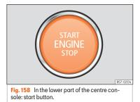
The engine can be started with a start button (Press & Drive). To do so, there must be a valid key inside the vehicle in the area of the front or rear seats, or on the centre console.
