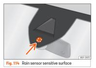
The rain sensor controls the frequency of the windscreen wiper intervals, depending on the amount of rain  $\gg \Delta$ . The sensitivity of the rain sensor can be adjusted manually. Manual wipe  $\gg$  page 128.
