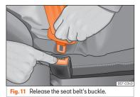
Properly worn seat belts hold the vehicle occupants in the position that most protects them in the event of an accident or sudden braking  $\mathfrak{M}$ .
