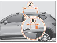
**Fig. 139** Attachment points for the roof railings for the roof carrier system.
