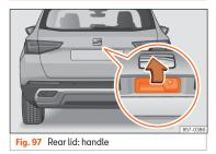
The rear lid opening system operates electrically. It is activated by exerting slight pressure on the handle **>>> Fig. 97**.
