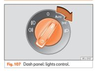
• Turn the switch to the required position **>>> Fig. 107**.
