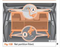
The purpose of the net partition is to prevent the items in the boot from moving into the cabin, e.g. in the event of sudden braking.
