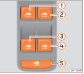
**Fig. 103** Detail of the driver's door: window controls.
