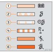
Fig. 212 On the inside of the cover of the battery charging socket: sticker with information on the charging process display.
