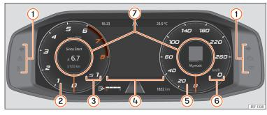
Fig. 60 Conventionally powered vehicles: SEAT Digital Cockpit on the instrument panel (classic view).
