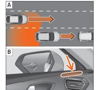
Fig. 190 Schematic representation: A Passing situation with traffic behind the vehicle. B Indication of the lane departure warning in the control lamp on the left side.
