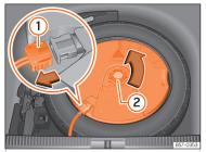
**Fig. 238** In the luggage compartment: remove the subwoofer.
