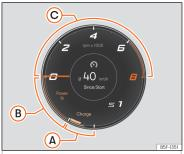
Fig. 65 Digital instrument panel: Power meter
