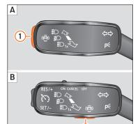
Fig. 72 On the turn signal and main beam lever: button for driver assistance systems (depending on versions).
