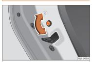
Fig. 91 Childproof lock on the left hand side door.
