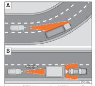
**Fig. 182** A Vehicle on a bend. B Motorcyclist ahead, out of range of the radar sensor.
