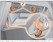
**Fig. 50** glove compartment (right hand drive): fuse box access.
