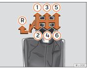
Fig. 161 Gear shift pattern of a 6-speed manual gearbox
