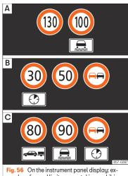
**Fig. 56** On the instrument panel display: examples of speed limits or overtaking prohibitions with their respective additional signs.
