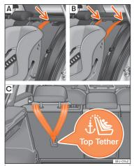
Fig. 28 Side seats of the second row: adjustment and assembly according to the Top Tether belt.
