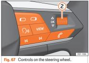
The steering wheel includes multifunction modules from where it is possible to control the audio, telephone, navigation, voice con-
