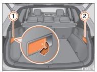
Fig. 112 In the luggage compartment: levers for release, from the luggage compartment, of the left part ① and right part ② of the rear seat backrest. The rear seat backrest is split and each part can be lowered forward separately to extend the luggage compartment.
