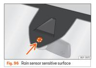
The rain sensor controls the frequency of the windscreen wiper intervals, depending on the amount of rain »» A. The sensitivity of the rain sensor can be adjusted manually. Manual wipe »» page 121.
