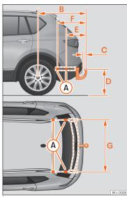
Fig. 216 Limits and attachment points for retrofitting a towing bracket.
