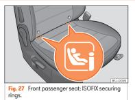
the rings are secured to the seat frame. The "ISOFIX" rings are located between the backrest and the seat cushioning of the rear seat **>> Fig. 26** and of the front passenger seat **>> Fig. 27**.
