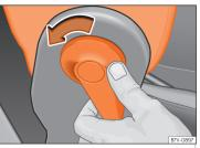
Fig. 110 Unlocking the folding backrest of the front passenger seat
