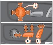
Fig. 100 Driver's seat: electric seat settings.
