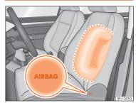
Fig. 21 Side airbag in driver's seat.
