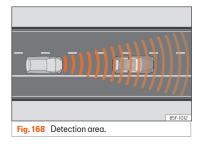
A radar sensor may be fitted to the front bumper of the vehicle **>>> Fig. 167**. The front radar detects any objects in its detection zone **>>> Fig. 168** and provides support for the following functions:
