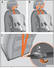
Fig. 29 Front passenger seat: adjustment and assembly according to the Top Tether belt.
