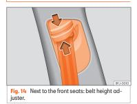
Using the height adjusters for the front seats and the outer seats of the second row, the position of the seat belts can be adjusted in the shoulder area according to the height of the occupant:
