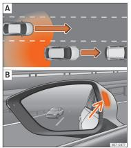
Fig. 191 Schematic representation: A Passing situation with traffic behind the vehicle. B Indication from the blind spot detector in the lefthand external mirror.
