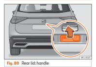
The rear lid opening system operates electrically. It is activated by exerting slight pressure on the handle **>>> Fig. 80**.
