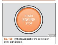
The engine can be started with a start button (Press & Drive). To do so, there must be a valid key inside the vehicle in the area of the front or rear seats, or on the centre console.
