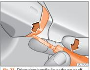
Fig. 77 Driver door handle: lever the cover off
