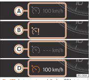
Fig. 173 Instrument panel display: GRA status indications.
