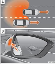
Fig. 192 Schematic representation: A Situation of passing and then moving into the righthand lane, B Indication from the blind spot detector in the right-hand external mirror.
