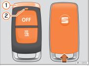
Fig. 149 Auxiliary heating: radio-operated remote control.
