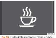
Fig. 55 On the instrument panel display: driver alert system symbol.
