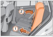
Fig. 102 Rear seat backrest adjustment.
