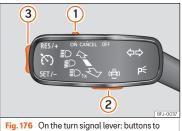
Fig. 176 On the turn signal lever: buttons operate the speed limiter.
