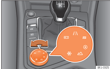
170. att. Viduskonsole: grozāmā poga (Driving Experience button).
